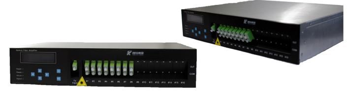
GAD series is a low noise, high performance, FTTP high power, multi-ports optical amplifier with gain spectrum band within 1540~1563nm. Each output port for optical amplifier has built-in well-performed CWDM. Every external up-link optical port of optical amplifier can connect with OLT PON port very conveniently. Each 1550nm (CATV)'s output optical port multiplex 1310/1490n's data stream, in order to reduce the quantity of the component and improve the index and reliability of the system.
